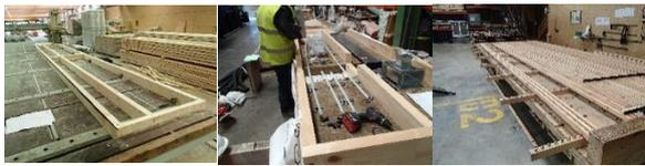
Figure 3: Manufacturing process of the modules.
